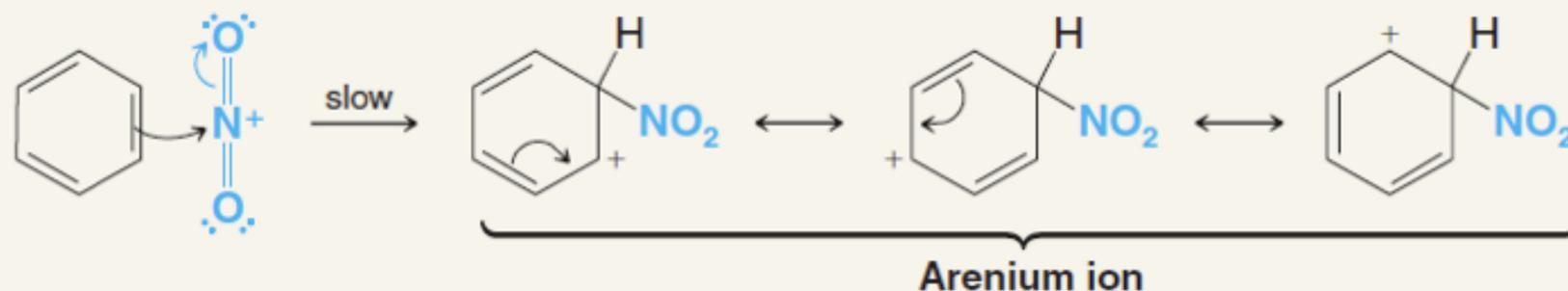
The nitronium ion is the electrophile in nitration; it reacts with benzene to form a resonance-stabilized arenium ion.
